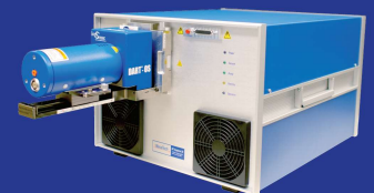
MT Explorer 50 Field-Deployable Tandem MS with DART Ion Source
