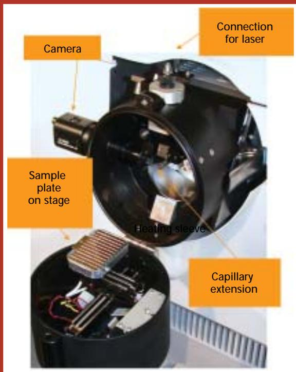
**Figure 2.** Ion trap MS fitted with an AP-MALDI source. The source chamber, which remains at atmospheric pressure, is shown in its open position to expose the inner workings. The sample plate, with positions for 96 samples, is mounted on a movable stage on the left half of the source. When the chamber is closed, the stage moves the plate
