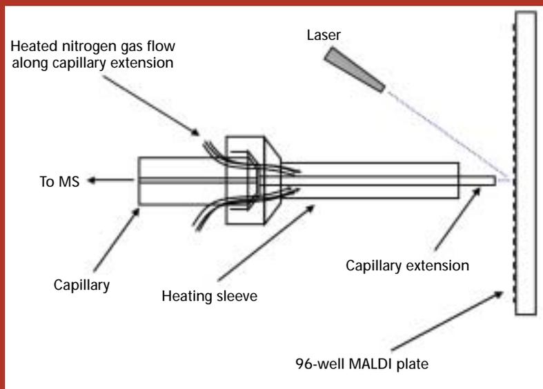
**Figure 1.** Schematic of the AP-MALDI source. Sample and co-crystallized matrix are desorbed from the 96-spot target plate using a pulsed 10-Hz nitrogen laser beam (337 nm) incident at an approximately 45° angle to the plate. Resultant gas-phase ions are drawn into the capillary extension, while admission of low-mass matrix clusters is minimized by using a heated nitrogen gas flow around the capillary extension, countercurrent to the ion beam.
