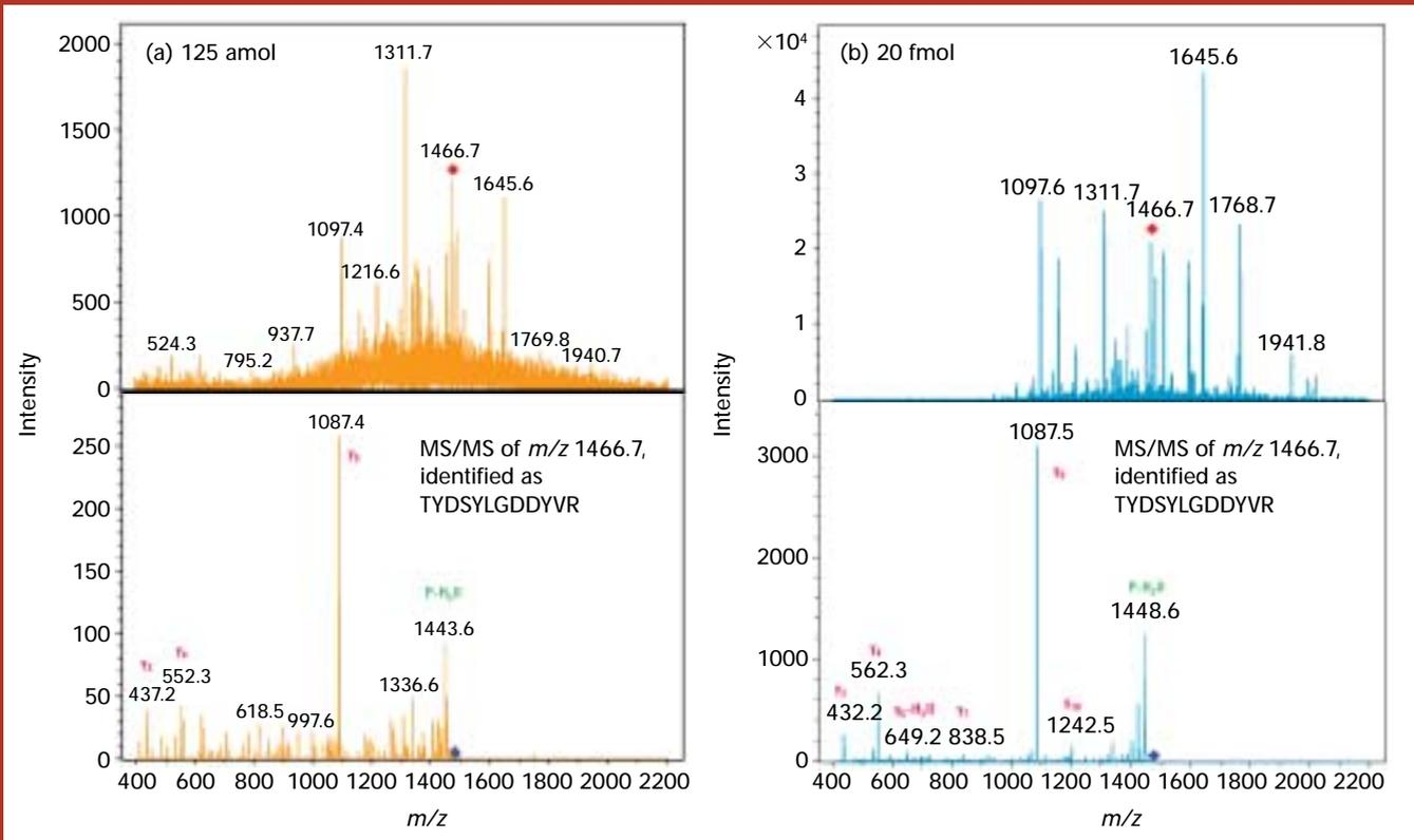
**Figure 3.** High-sensitivity MS-MS analysis. Shown here are the MS and MS-MS spectra of a commercially available tryptic digest of bovine apotransferrin obtained by analyzing 125 amol (left) and 20 fmol (right). The resemblance is obvious despite the 160-fold difference in amount. The product ion spectra of  $m/z = 1466.7$ , selected automatically during MS-MS operation, are shown. Several diagnostic b- and y-series ions can be identified.
