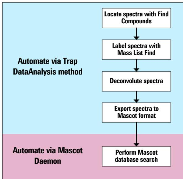
**Figure 13** Data analysis with the LC/MSD Trap software and Mascot search
