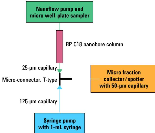
**Figure 10** Schematic for micro fractionation/spotting with online matrix addition
