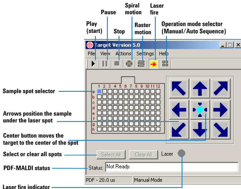
**Figure 6** Main Target program screen
