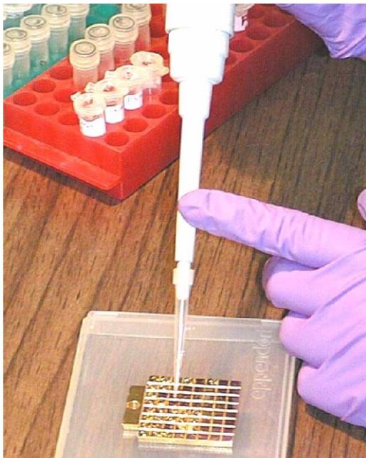
**Figure 3** Spotting samples: best arm position and distance from plate
