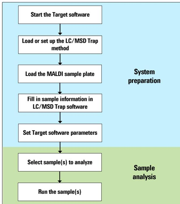
**Figure 5** MALDI MS/MS procedure
