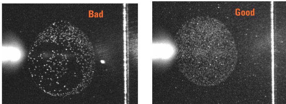
**Figure 11** A bad LC MALDI spot formed when the contact control distance was set too low, and a good spot shown after increasing this distance
