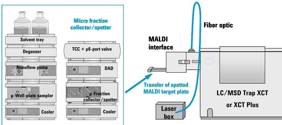
**Figure 9** Micro fraction collector/spotter and interface to MALDI MS/MS system
