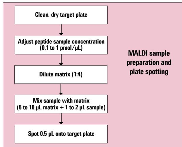
**Figure 2** Procedure for MALDI sample preparation
