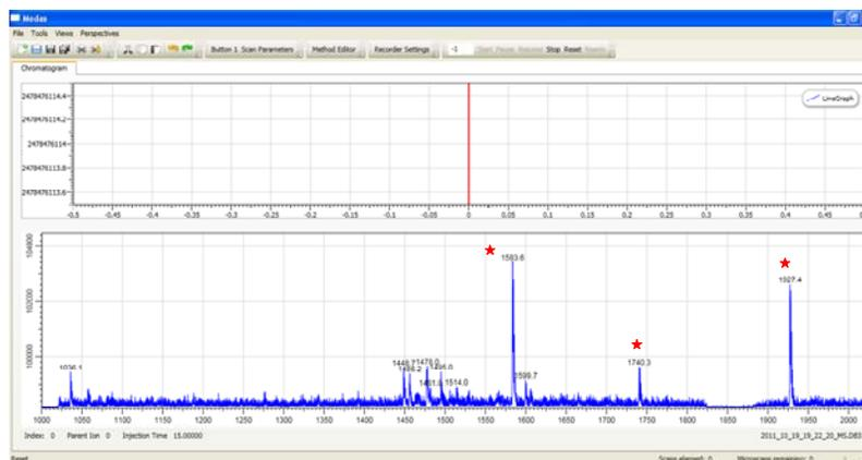
Figure 4: AP MALDI MS spectrum of *Bacillus globigii* spores ( $3 \cdot 10^6$  cfu) after chemical processing and digestion by trypsin. *Bg* spores biomarker peptides are indicated.
