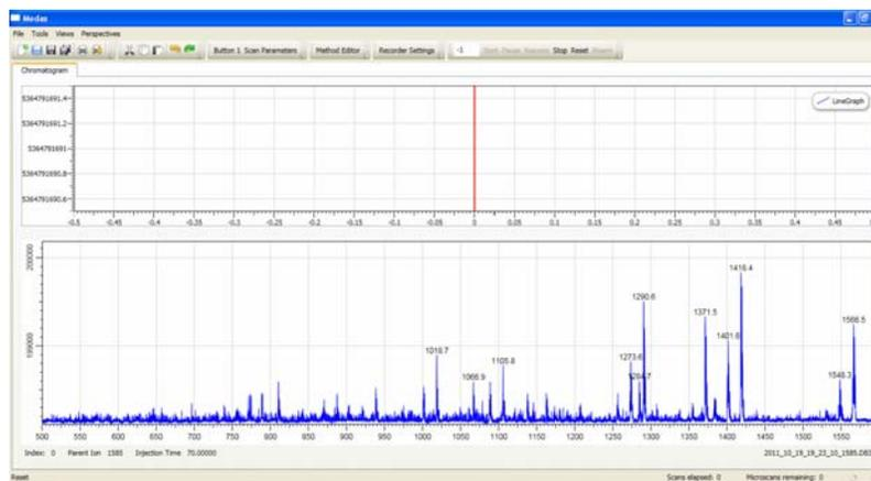
Figure 5: AP MALDI MS/MS spectrum of peptide ion with m/z value of 1584 in Figure 4.
