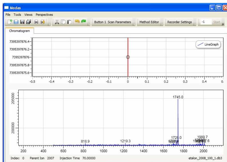
Figure 3: AP MALDI MS/MS spectrum of peptide ion with  $m/z$  value of 2008 in Figure 2.
