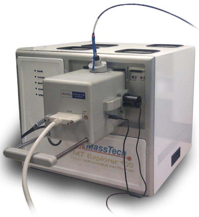
Figure 1: AP MALDI PDF<sup>+</sup> ion source coupled to MT Explorer 100 MS.
